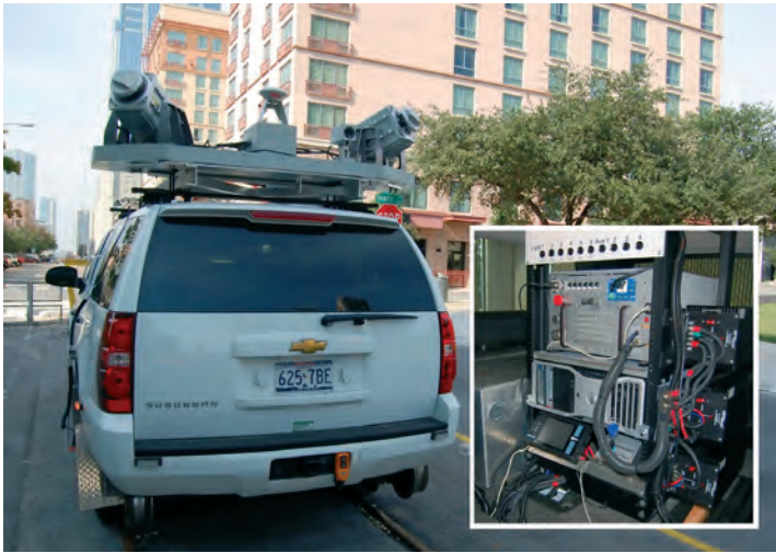
▲ SAM's mobile Lidar vehicle and equipment.
