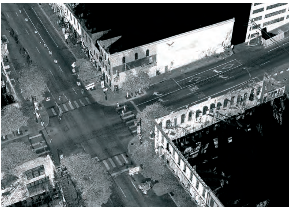
◀ Lidar point clouds showing street intersections and building facades.
